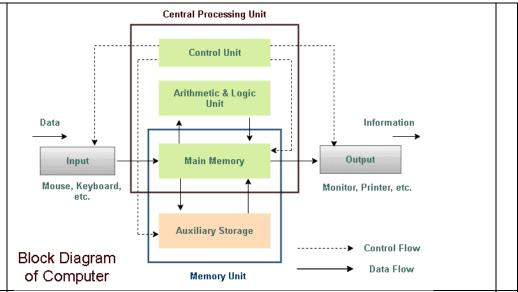
The block diagram represents how data and instructions flow between the CPU, memory, and I/O devices, managed by the Control Unit. In simple terms, a Block Diagram of a Computer helps us understand how a computer works, from collecting input data, processing & formatting the data, and generating the output results in the way user commands. The computer system consists of three main parts: Input Units, CPU, and Output Units
