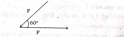
Two forces, each equal to F act on the shown figure, determine Resultant:
