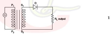
During the half cycle diode D is forward biased and forward current flows through the diode; we get output. During –ve half cycle diode D will be reverse biased hence will not conduct. The output waveform is shown in fig. 1
