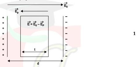
Let  $C_0 = \frac{A\varepsilon_0}{d}$  be capacitance of capacitor with air between the plates.
