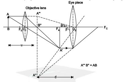
Magnifying power of compound microscope is defined as ratio of angle subtended by final image and object on eye when both are at least distance of distinct vision.
