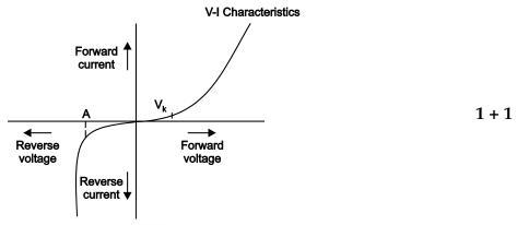
**Breakdown voltage :** It is the reverse voltage at which the breakdown of junction takes place and reverse current increases rapidly. It is shown by the region *OA*. If reverse current increases the safest rated value of diode then it will get damaged.
