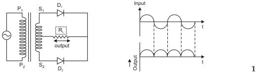
During +ve half cycle diode  $D_1$  is forward biased and diode  $D_2$  is reverse biased. The forward current flows due to  $D_1$ . During –ve half cycle, diode  $D_1$  is reverse biased and
