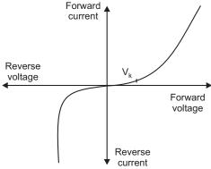
It is found that beyond forward voltage  $V = V_K$  called knee voltage, the conductivity is very high. Potential barrier is overcome and the current increase rapidly.
