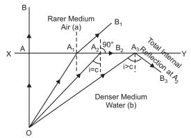
Optical fibres are the threads of glass or quartz of ref. index 1.5 coated with a thin layer of material having low ref. index nearly 1.48.
