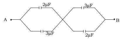
Calculate the net capacitance between A and B in the given network.
