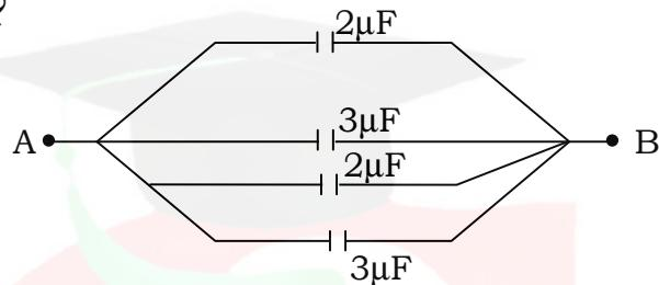
Calculate the net capacitance between A and B
