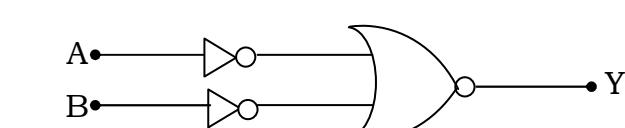
Write the truth table for the circuit shown in the following Figure. This circuit acts like which gate ?
