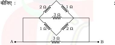
Calculate the equivalent resistance between the points A and B in the given Figure :
