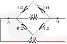
Calculate the equivalent resistance between the points *A* and *B* in the given Figure.
