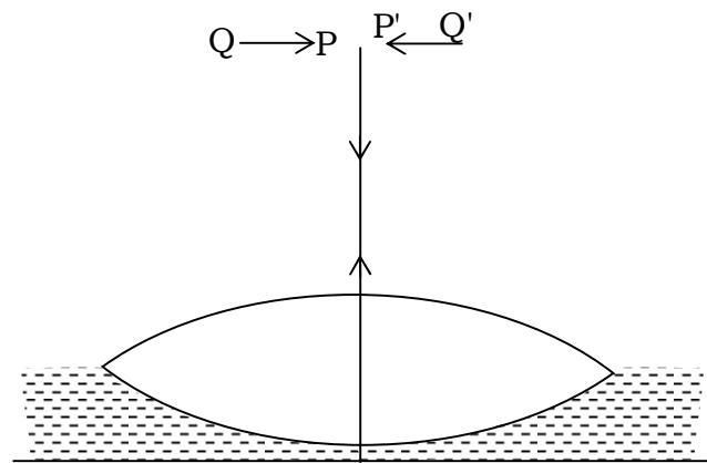
Fig. shows an equiconvex lens (of refractive index 1.50) in contact with a liquid layer on top of a plane mirror. A small needle with its tip on the principal axis is moved along the axis until its inverted image is found at the position of the
