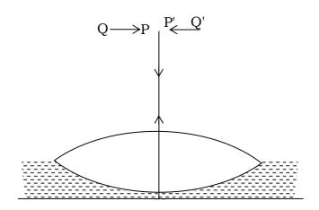
Fig. shows an equiconvex lens (of refractive index 1.50) in contact with a liquid layer on top of a plane mirror. A small needle with its tip on the principal axis is moved along the axis until its inverted image is found at the position of the needle. The distance of the needle from the lens is measured to be 45 cm. The liquid is removed and the experiment is repeated. The new distance is measured to be 30 cm. What is refractive index of the liquid?
