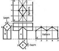
To develop the pattern of t pipe, what should be the angle used?
